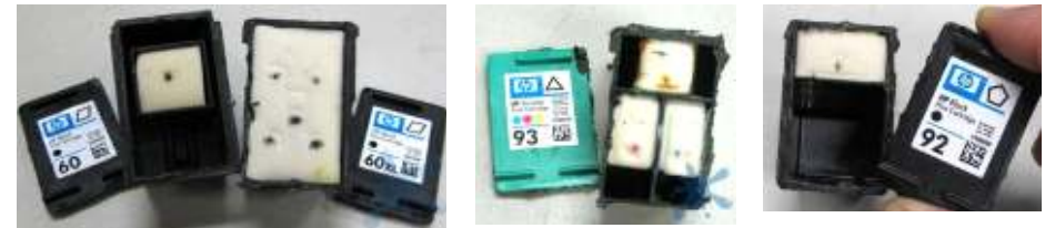
Above pictures show different internal sponge designs used to force limited ink capacity in #60 black, #93 color, #92 black cartridges. Pictures below show large capacity sponge structure.
